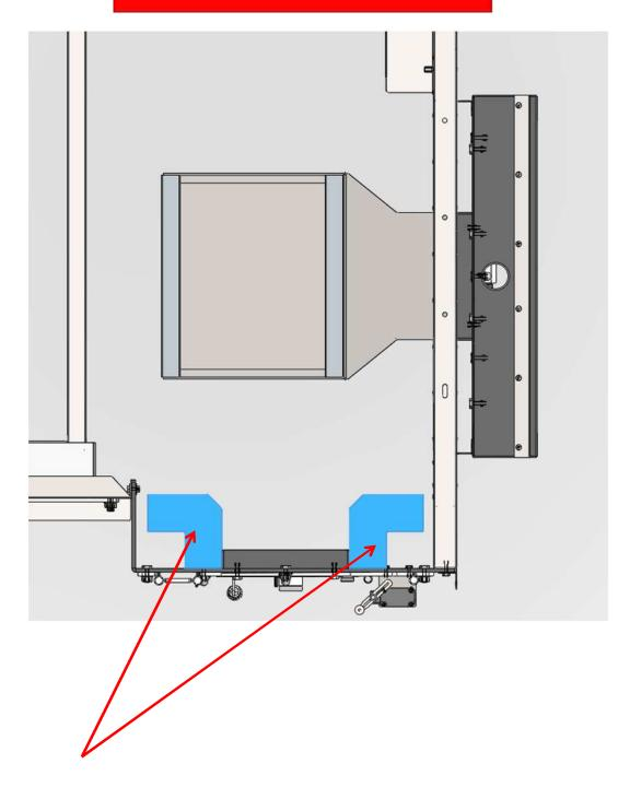
PLACE THE ANGULAR REFRACORY BRICKS WITH REFRACORY CEMENT CONTAINED IN THE BIN
