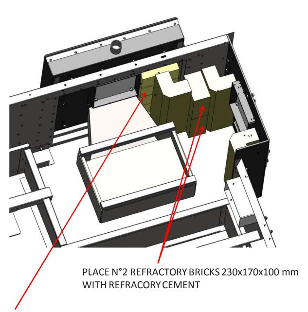
PLACE N°4 REFRACORY BRICKS 220x110x60 WITH REFRACORY CEMENT
