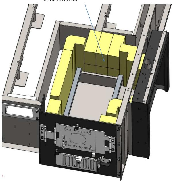
PLEASE NOTE : ALL THE BRICKS MUST BE FIXED WITH REFRACTORY CEMENT
