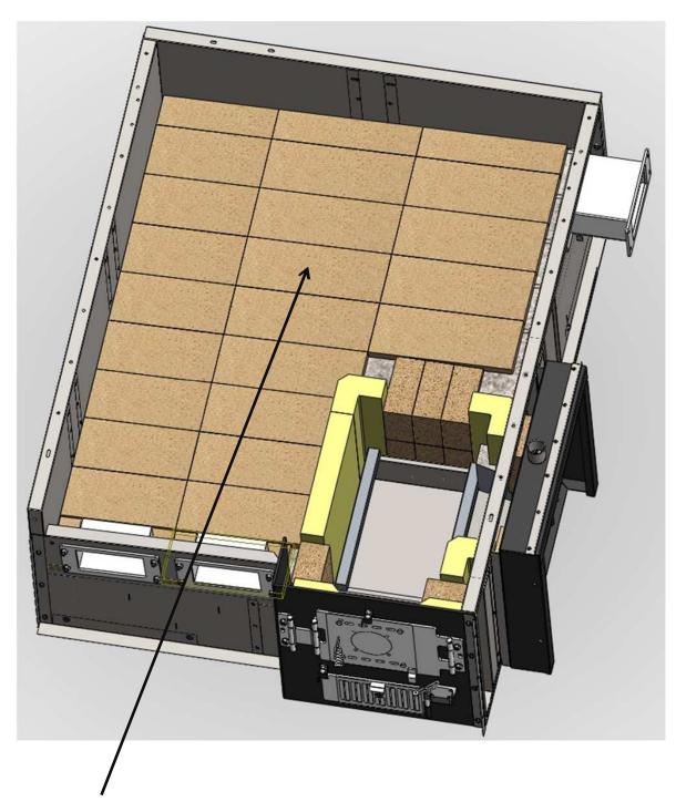
MAKE A FLAT LAYER WITH REFRACORY PLATES WITH MEASURE 500x200x30
