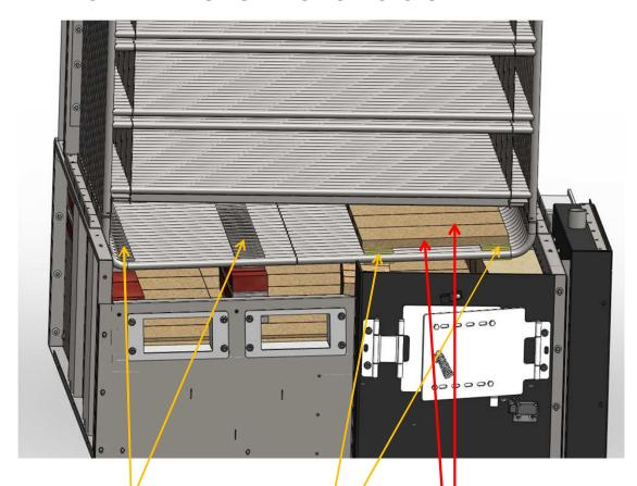
PLACE NORMAL CONCRETE BETWEEN THE TUBES
