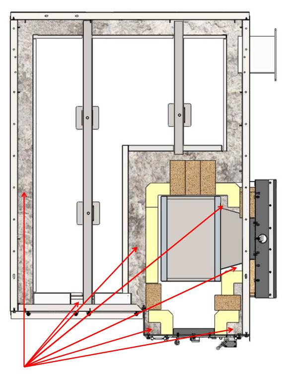
FILL WITH NORMAL CONCRETE UNTIL THE HEIGHT OF THE RECTANGULAR TUBES
