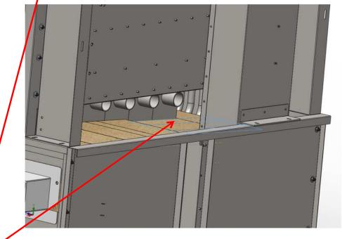
COVER THE OPEN PART OF CHANNELS WITH REFRACORY PLATES 500x200x30
