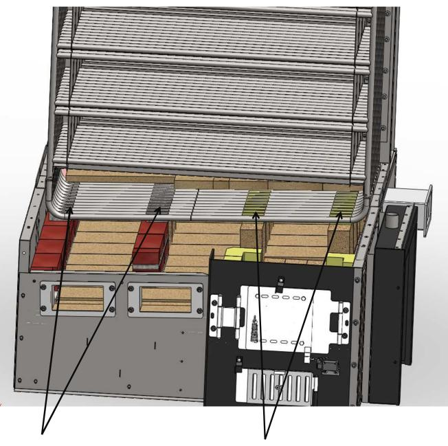
FILL WITH NORMAL CONCRETE BETWEEN THE TUBES
