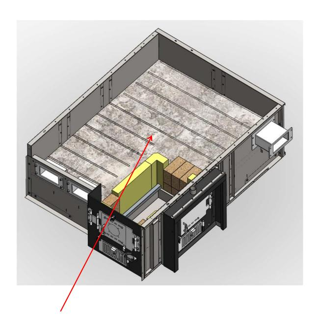
MAKE A LAYER OF NORMAL CONCRETE UNTIL REACHING THE LEVEL OF FOLDS
