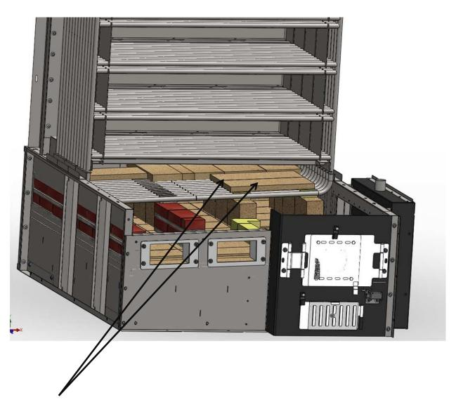
PLACE N°2 REFRACORY PLATES 500x200x30 FOR CLOSURE OF FIRST REFRACTORY CHANNEL
