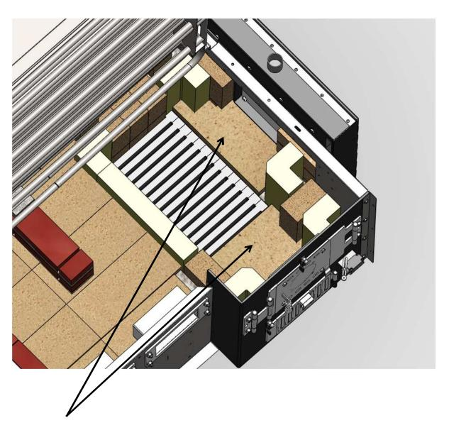
MAKE TWO INCLINED PLANS WITH REFRACTORY PLATES 500x250x40 THAT MUST BE CUT IN LOCAL SITE
