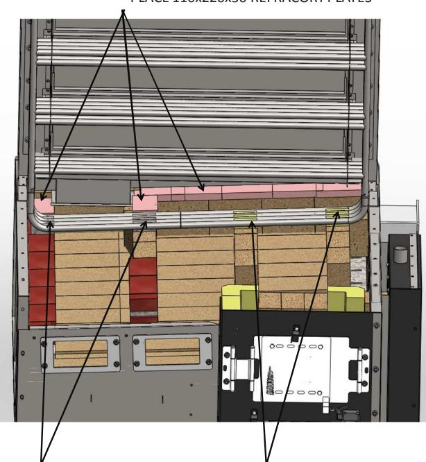
FILL WITH NORMAL CONCRETE BETWEEN THE TUBES
