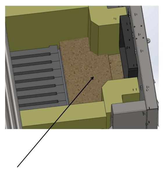
MAKE ONE INCLINED PLANS WITH REFRACTORY PLATES 500x250x40 THAT MUST BE CUT IN LOCAL SITE
